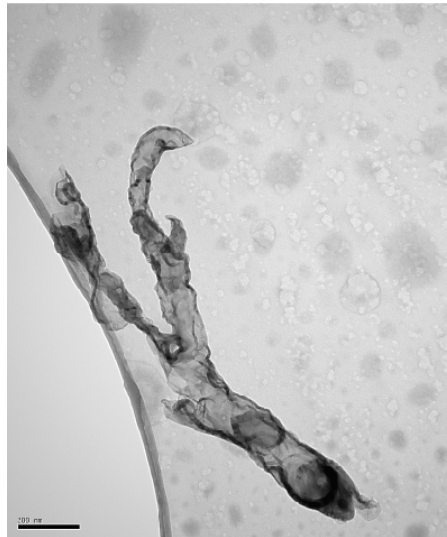
Fig.5 TEM image of a Y-shaped BSA nanotube (The scale bar is 200nm.)
