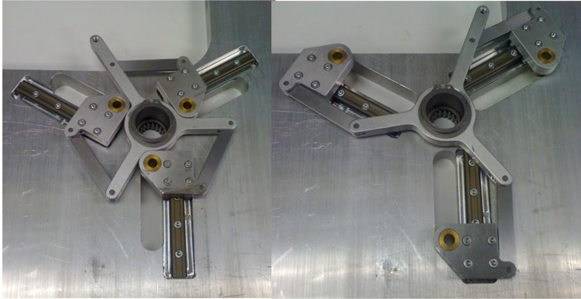
Figure 3.14: Finished control linkage
