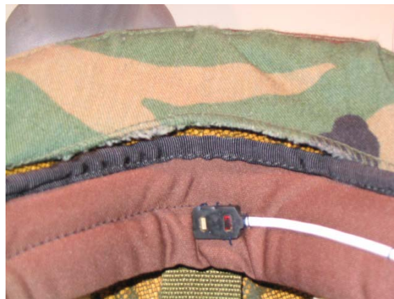
Figure 4.8. Securing the sensor to the inner lining of a helmet for attachment to the forehead.
