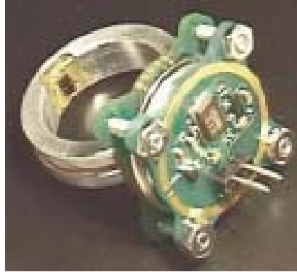
Figure 2.11. Transmission mode finger-ring sensor for reduction of pressure effects [63].
