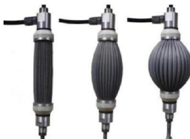
Fig. 1.6: The state of Mckibben muscle as it is pressurized
