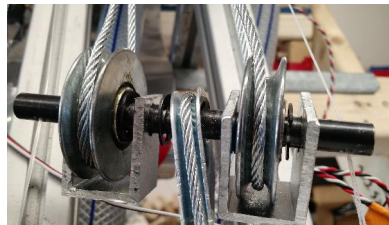
Fig 4.9: The final force multiplier design employing free hanging pulleys
