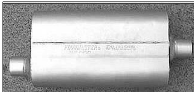
Fig. 23. Case 2 – Flowmaster brand 40 series muffler (Flowmaster, Inc., 2009).
