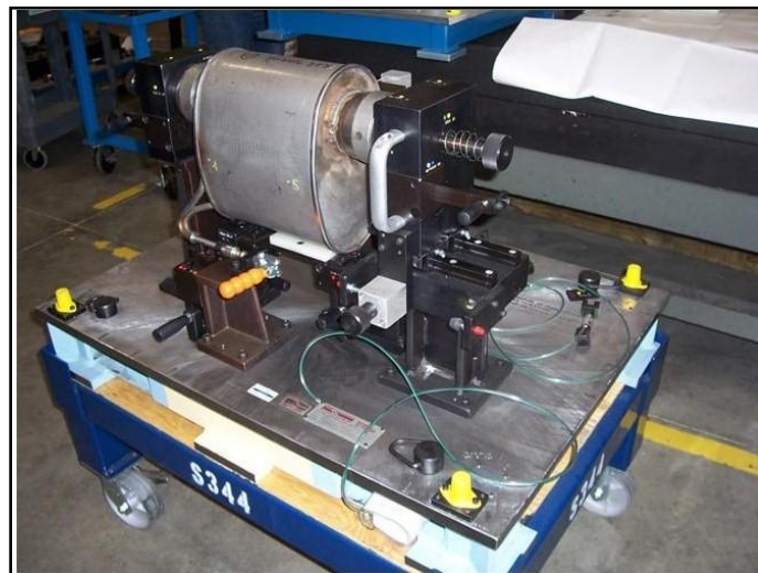
Fig. 20. First example of a dedicated muffler welding fixture (Peterson Jig and Fixture, 2007).
