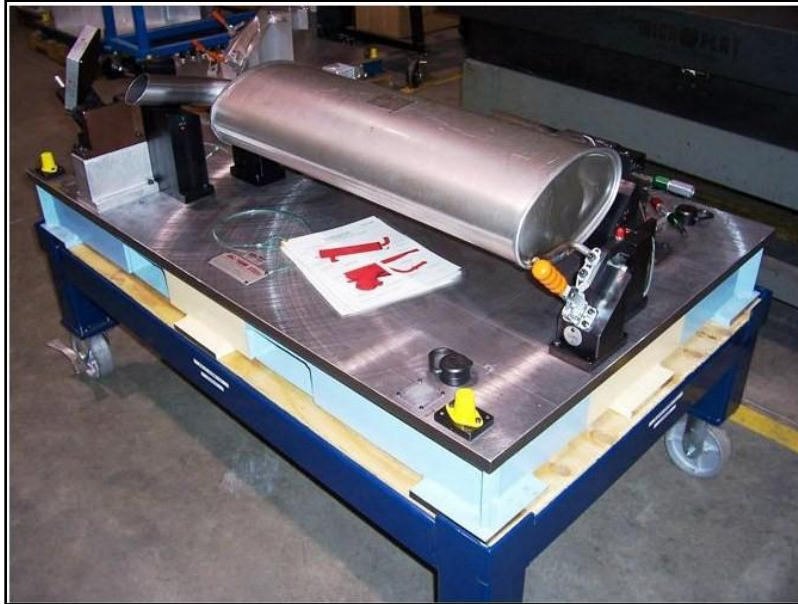
Fig. 21. Second example of a dedicated muffer welding fixture (Peterson Jig and Fixture, 2007).
