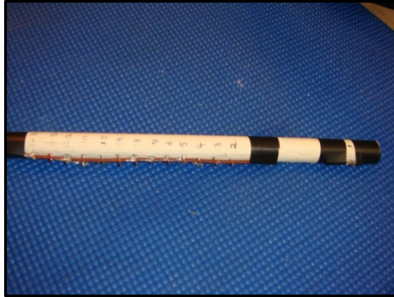
Figure 6.5 Thermocouple tree consisting of 15 J type thermocouples
