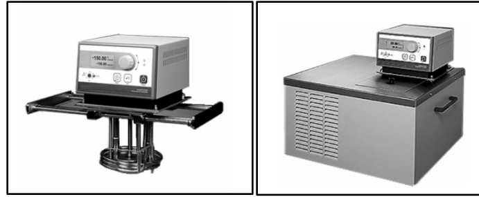
Figure 6.3 Circulation pump / heater (left), circulation bath (right)
