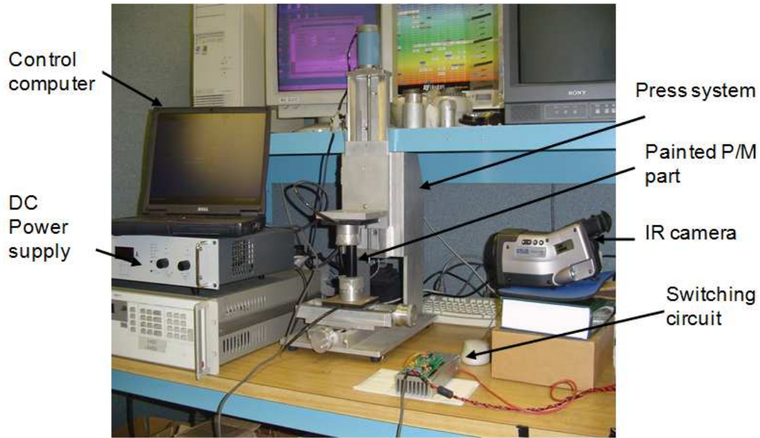
Figure 6.8: Picture of the pulsed DC setup.
