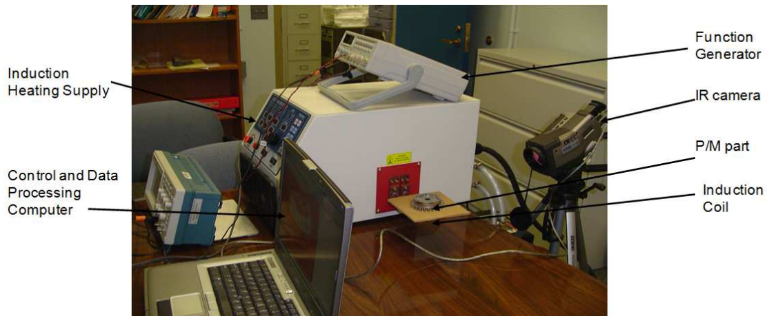
Figure 6.19: Picture of the pulsed induction system.
