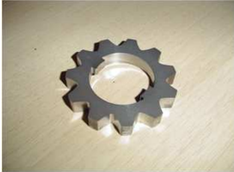
Figure 6.22: Green state P/M compact (part courtesy of Nichols, Portland, ME).
