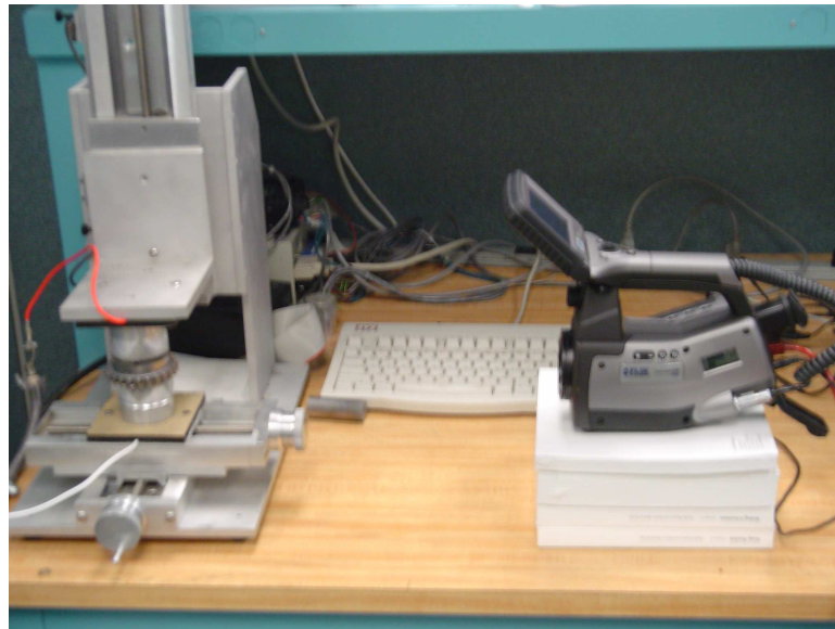
Figure 6.2: Generic test arrangement showing the electrode contacts.
