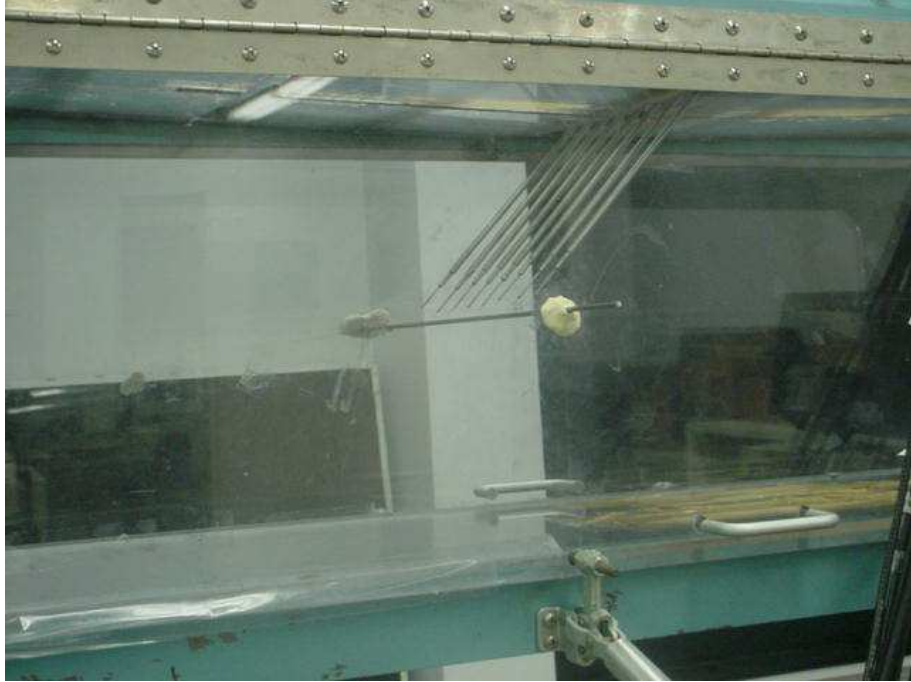
Figure 5.1: Diagram of the experimental setup for velocity measurement.
