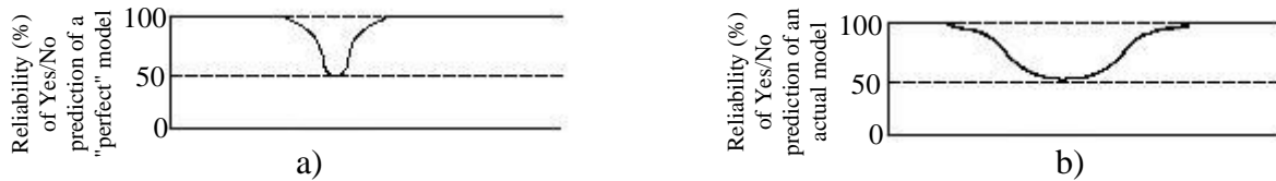
Figure 1: Reliability of the predictive capability of a model to clearly state "yes or no" to an engineering question, as a function of single input parameter values, a) for a "perfect" model and b) for an actual model [6]
