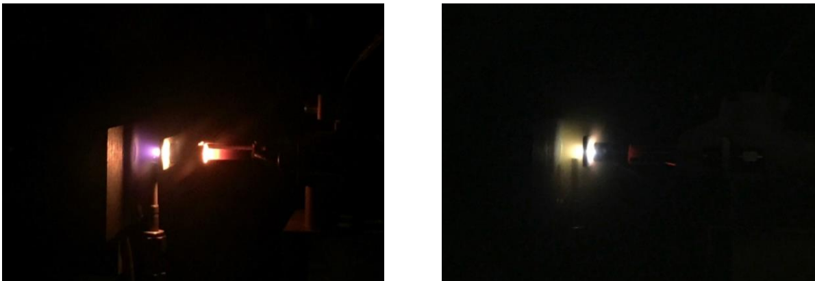
Figure 71: BaO hollow cathode in operation on xenon (left) and iodine (right).
