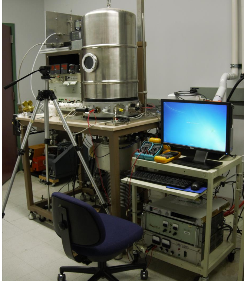
Figure 37: Vacuum facility used for BaO cathode tests with iodine propellant.
