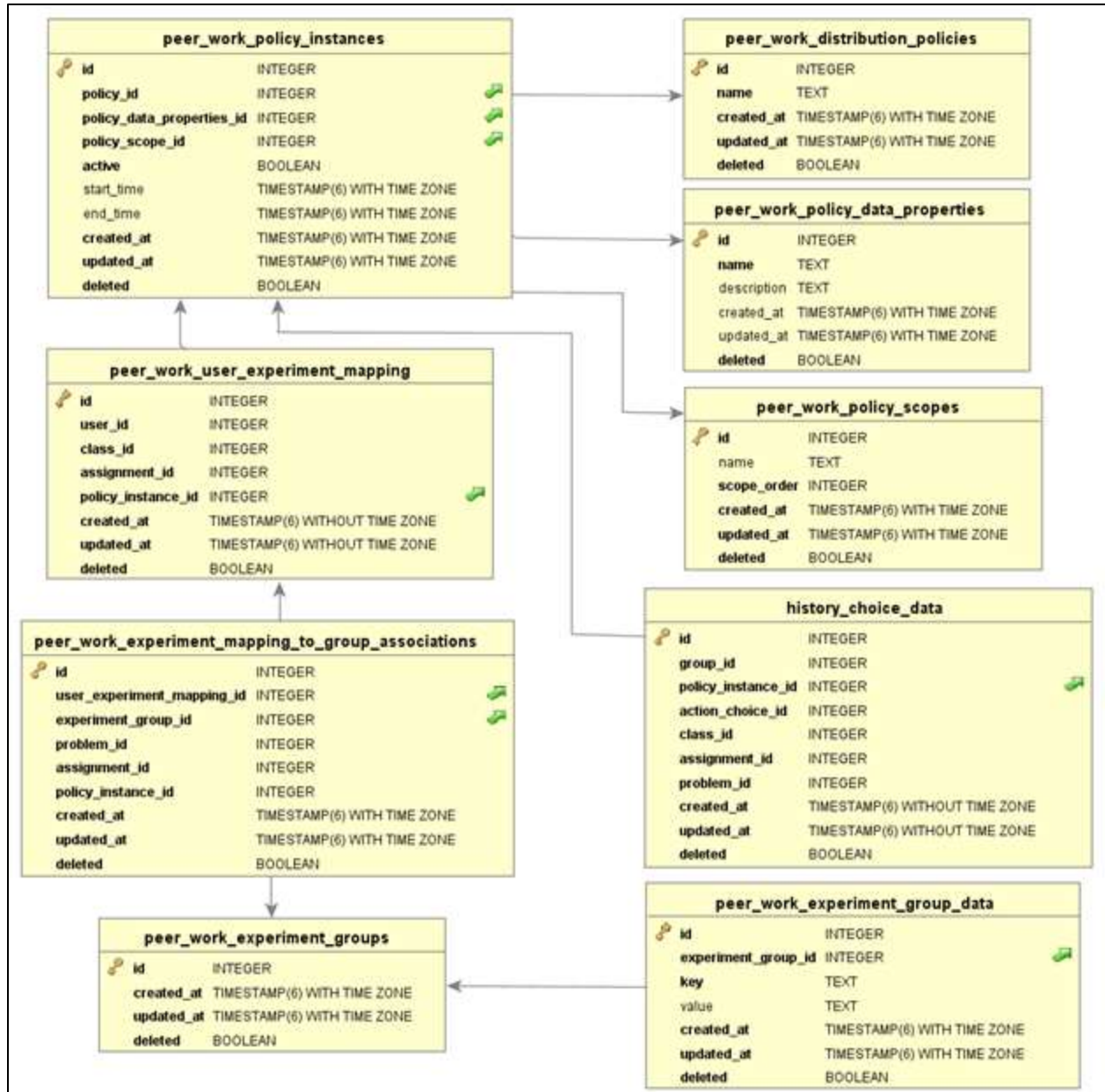
Figure 8.3.5.1. ER Diagram for the PeerASSIST database on tables related to the experiment infrastructure.
