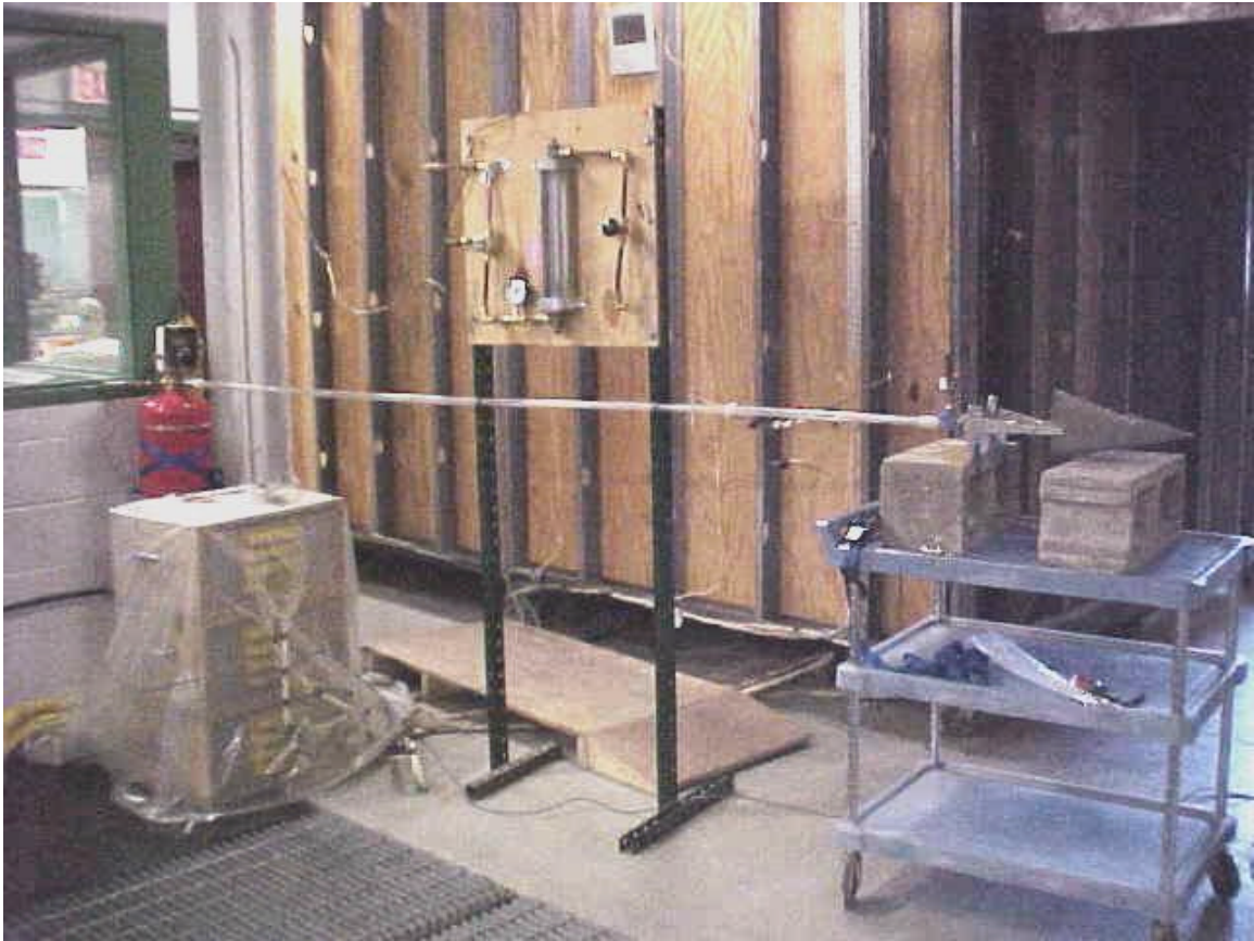
Figure 7.10 Cylinder-Pipe-Nozzle Test Configuration.
