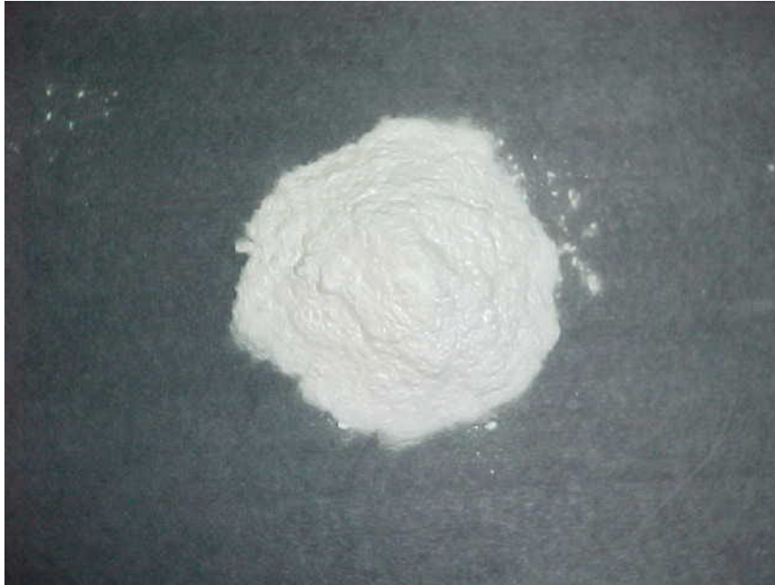
Figure 7.14 Sodium Bicarbonate Without Flow Additives.
