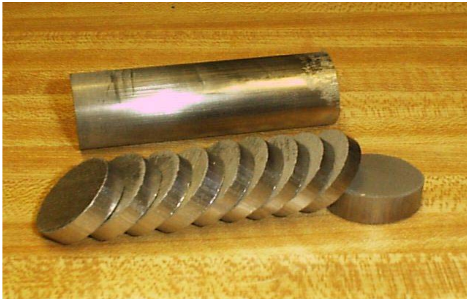
Figure 6.9: Green state P/M rod sliced into 0.25' thick pieces for density measurements.
