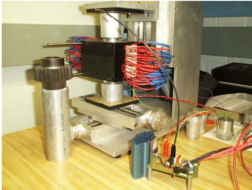
Figure 6.24: Measurement setup for EIT application to complex gear, showing the current source, bench press, sensor, and a part identical to the one that is currently in the sensor.
