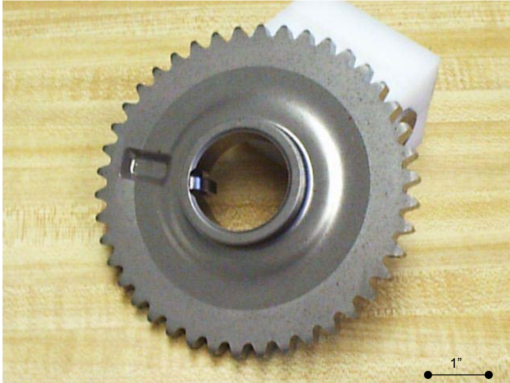
Figure 2.4: Complex, multi-level P/M part (courtesy of BorgWarner).
