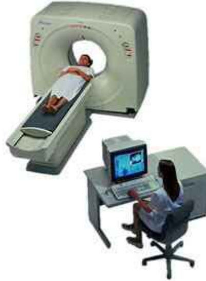
Figure 5.1: Medical X-ray CT system, which conducts scanning 2D projections and reconstructs 3D images.
