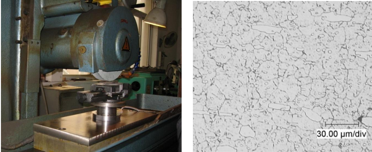
Figure 77 Experimental setup and the metallurgy structure of workpiece (D2)
