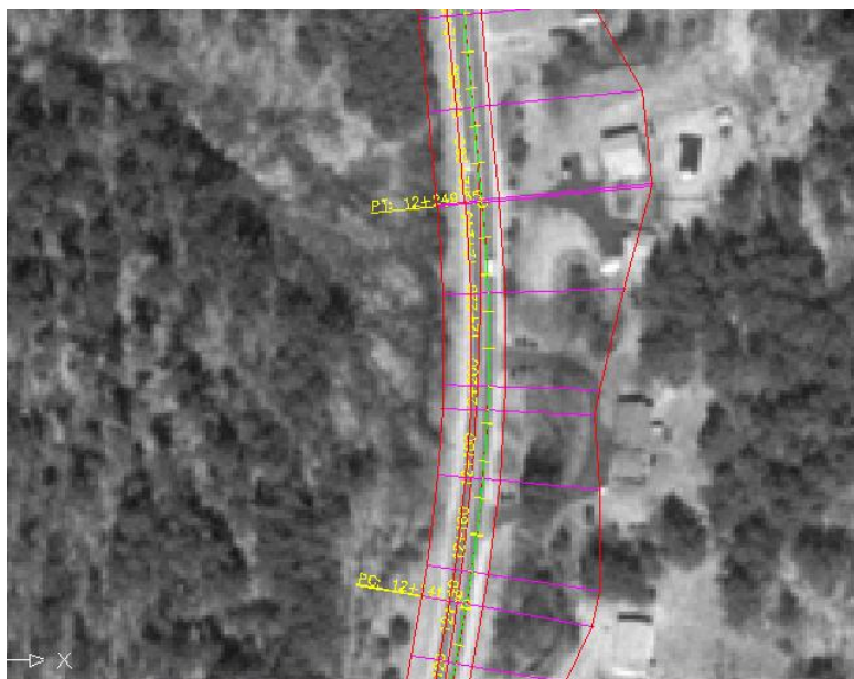
Figure 7-7. Impacts to Existing Residence STA 12+120 to 12+280.
