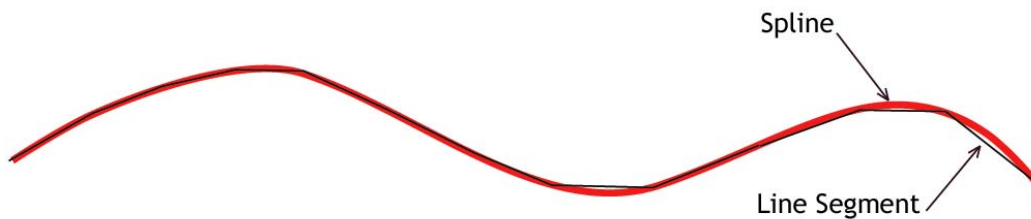
Figure 3.8: The same spline approximated with for line segments, corresponding to t values of 0, 0.25, 0.75 and 1.
