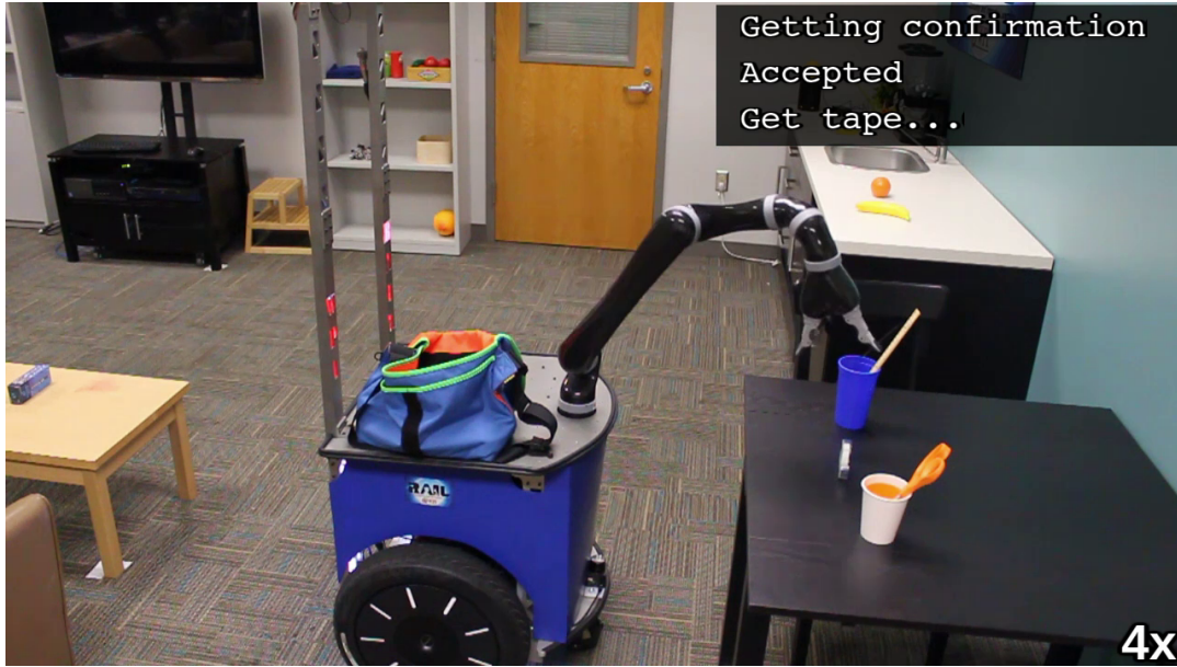
Figure 5.1: Screenshot showing the robot autonomously retrieving a roll of tape for the pack schoolbag task, after receiving user approval to use it instead of glue .
