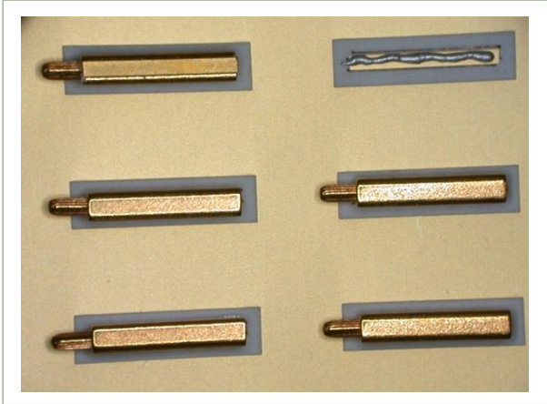
Figure 4-13. Batch process: quad line feed assembly
