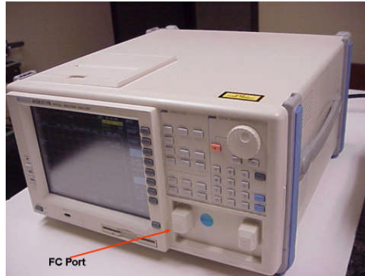
Figure B-2. Ando AQ6317B Optical Spectrum Analyzer located in the IPG Photonics Laboratory.
