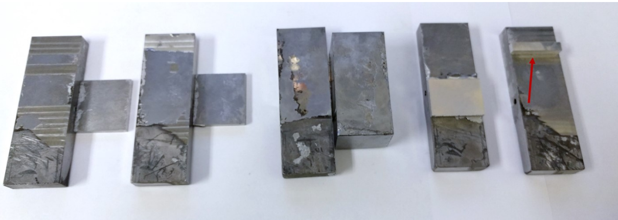
Figure 13: Machined shear samples with the red arrow indicating the only lug that stuck to the steel after machining operation finished.
