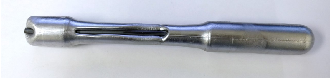
Figure 10: Incomplete filling due to the insert is blocking the flow of the molten aluminum.
