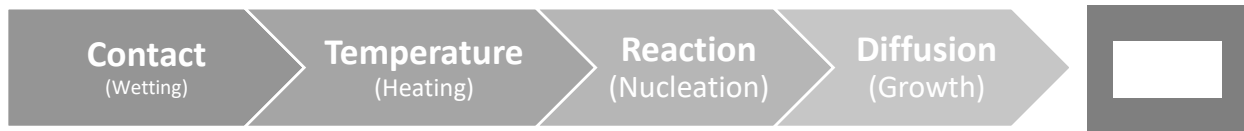
Figure 12: Steps in the metallurgical bond formation.
