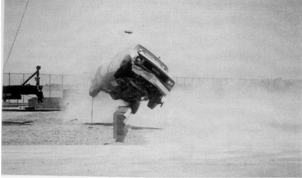
Figure 2.8: NCHRP Report 350 Test 3-11 impact with modified G4(1S) guardrail with nested 12-gauge w-beams and a 102-mm curb under the rail. (30)
