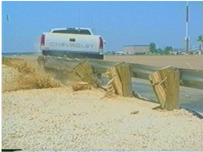
Figure 2.11: Guardrail damage in test TTI 404201-1. (32)
