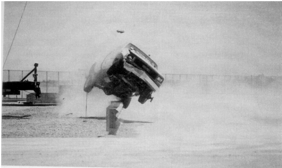
Figure 6.6: NCHRP Report 350 Test 3-11 impact with modified G4(1S) guardrail with nested 12-gauge w-beams and a 102-mm curb under the rail. (29)
