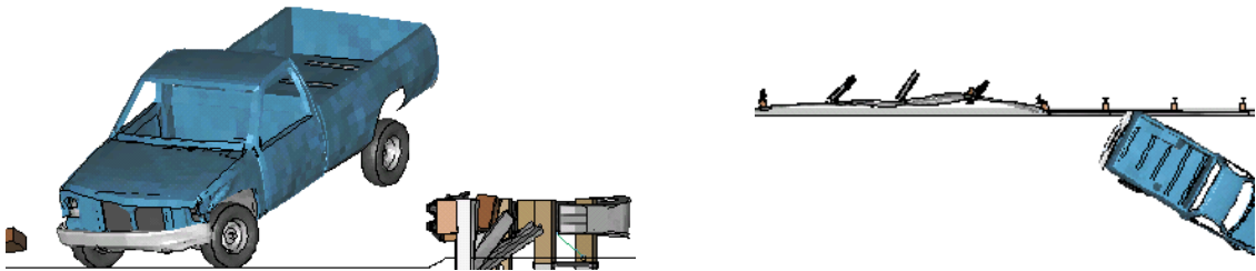
Figure H.9: (CONTINUED) Sequential views of curb-barrier impact from F.E. analysis - front view and top view Curb Type -- AASHTO G Curb Offset Distance -- 0m Impact Speed -- 100 km/hr Impact Angle -- 25 degrees.
