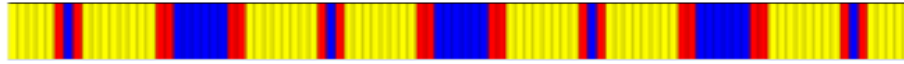
Figure 1: Approximation of three distinct layers – 100 wt% resin (yellow), 50-50 wt% resin and glass (red), and 100 wt% glass – in composite microstructure: Modified acrylic FRP with inorganic high-charring flame retardant additive
