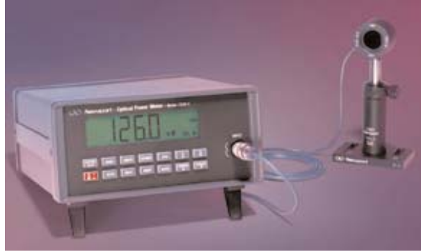
Fig. 4.16. Digital optical power meter used for experiments.
