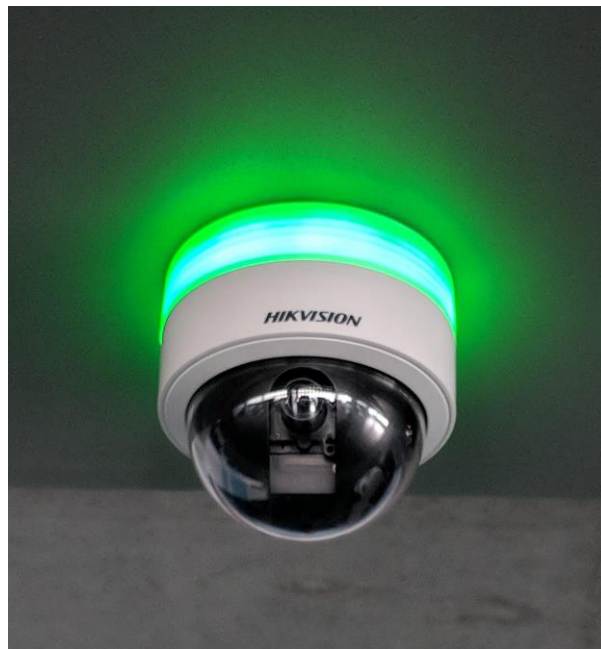
Figure 14: Jinhui OCR camera marking a vacant spot
