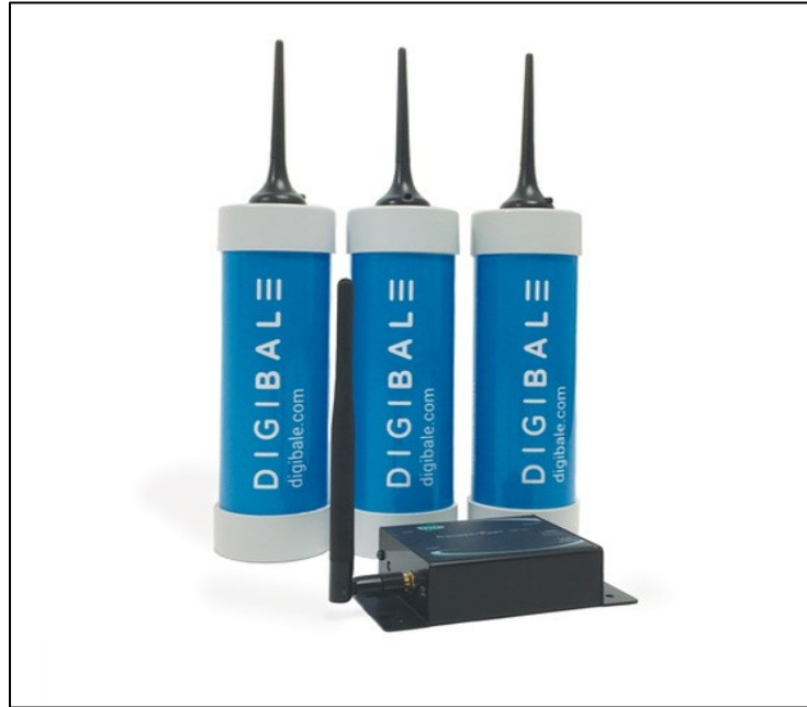
Figure 1. DigiBale Farm Automation Starter Kit with 3 sensor packages and a gateway.
