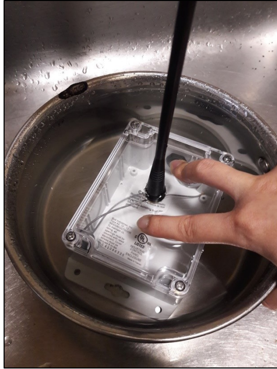
Figure 14. Waterproof Submersion Testing the Node
