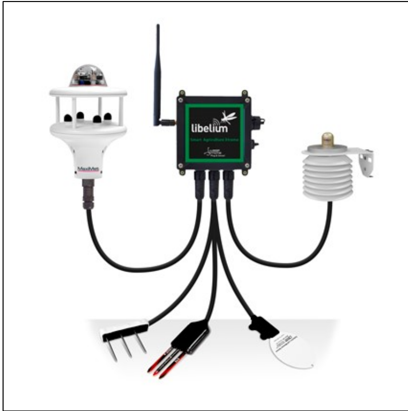
Figure 2 Libelium Smart Agriculture Xtreme sensor package
