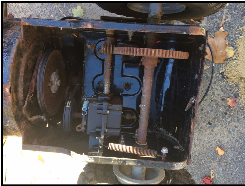
Figure 3: Undercarriage of the unmodified snowblower
