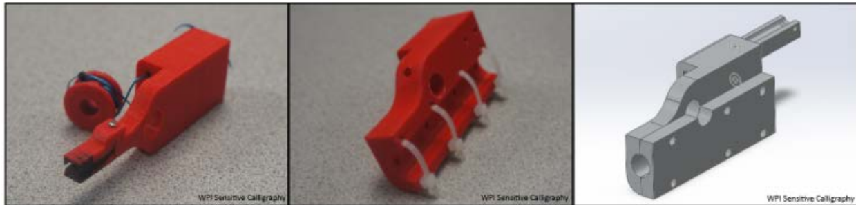
Figure 11: Three rejected prototypes. [LEFT] A prototype intended to hold a dip pen nib without a pen body. [CENTER] A prototype that held a fountain pen by the ad hoc usage of zip ties fed through an arched hole. [RIGHT] A prototype that clamps the pen into place with a plate attached via screws and has the linear potentiometer protruding off the back of the holder.
