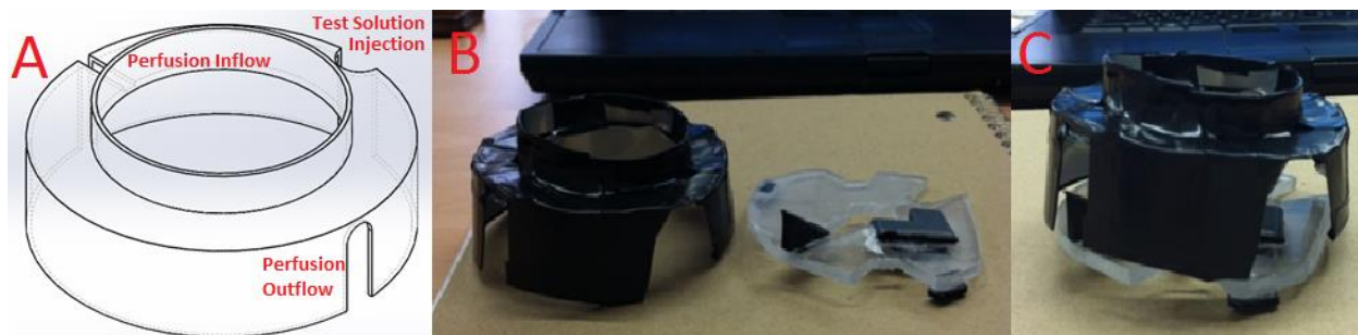
Figure 29: The light shield of prototype two; (A) computer model of the prototype two light shield, with various holes are cut into the sides to allow for the perfusion systems and the injection of the test solution, (B) the disk of prototype two and light shield, and (C) the assembled prototype two
