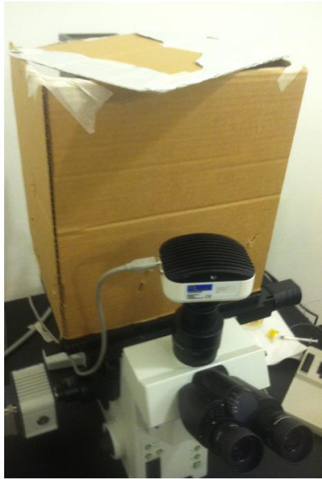
Figure 19: The cardboard box light shield; it completely blocks users from seeing or accessing the sample during imaging, but also blocks a large amount of ambient light from reaching the slide.
