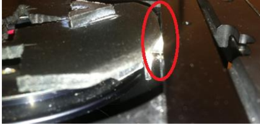
Figure 27: The interference of prototype one with the metal holder; prototype sits just on top of the holder, preventing a flush and consistent placement.
