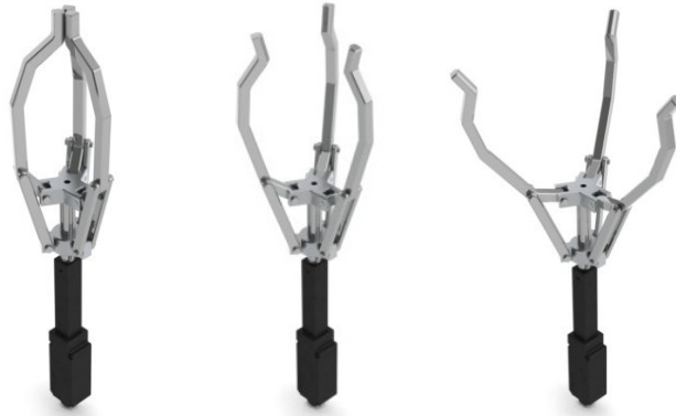
Figure 30: Inner Gripper Design Shown with Closed, Half and Full Open Configurations
