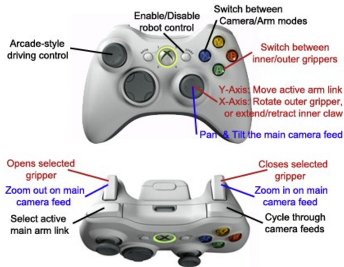
Figure 40: Gamepad Control Pin-out
