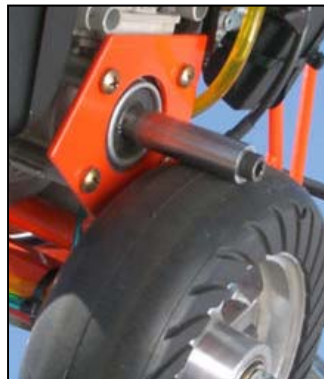
Figure 17: Friction Drive (Spindle Drive, 2009).
