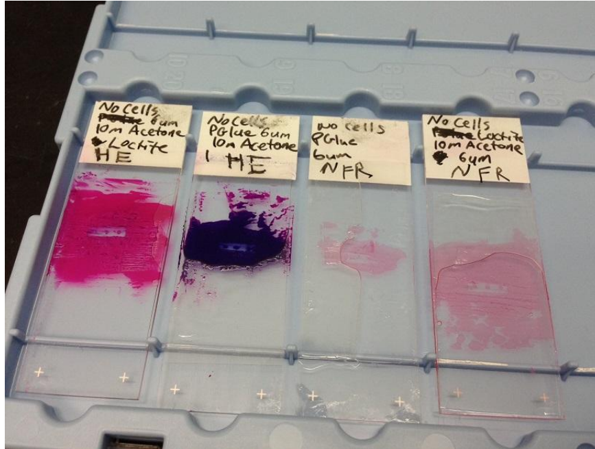
FIGURE 11: RESULTS OF GLUE TESTS ON EMPTY SCAFFOLDS. LEFT-RIGHT: H&E STAIN WITH LOCTITE, H&E STAIN WITH LIQUID NAILS, NFR STAIN WITH LIQUID NAILS, NFR STAIN WITH LOCTITE
