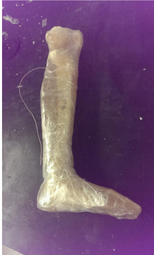
Figure 43 Ballistics gel leg model with suspended bone structures supported with plastic wrap
