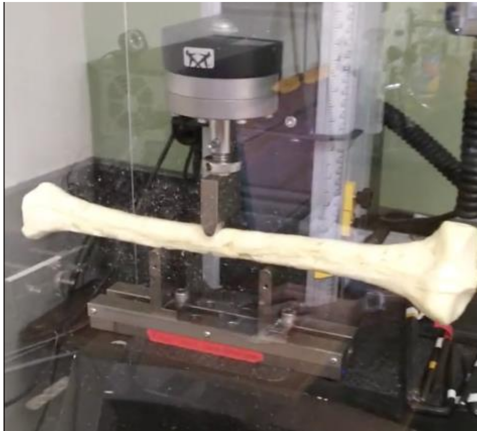
Figure 35 A SawBone set up in the Instron 5544
