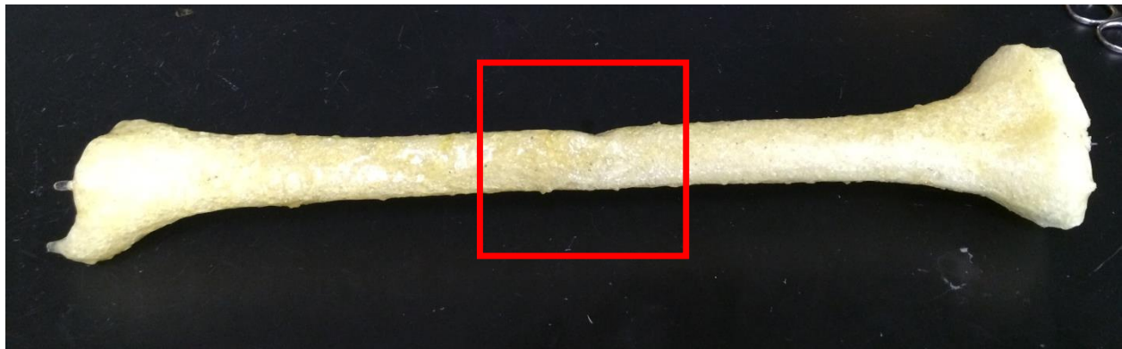
Figure 56 A high-density polyurethane bone after testing
