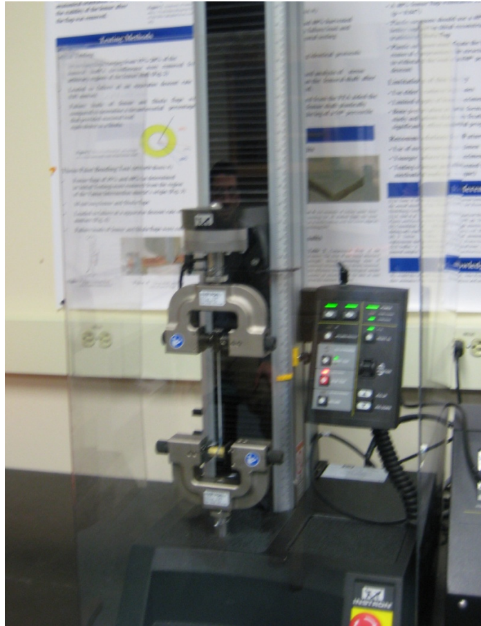
Figure 48: Glass shield placed around test set-up
