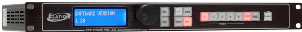
Figure 2 - 10: Elation Image VSC 2.0 Image processor used to condition video to be fed to a panel controller. From [16]
