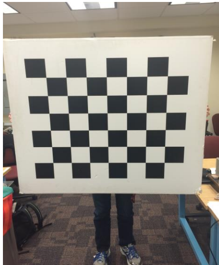
Figure 9: 7x5 Checkerboard Calibration Target
