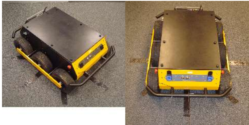
FIGURE 8: ANGLE TESTING SETUP - INITIAL POSE AND POSE AFTER 45 DEGREE ROTATION
