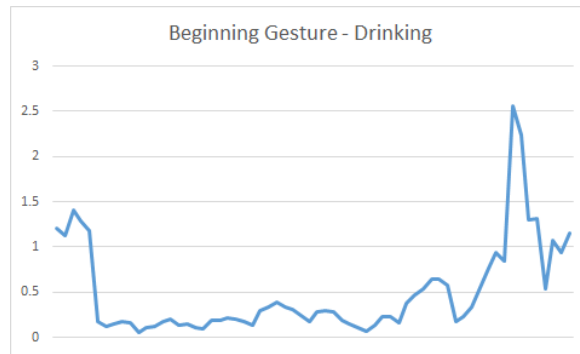
Figure 17 - Accelerometer Data of Start of Drinking Gesture
