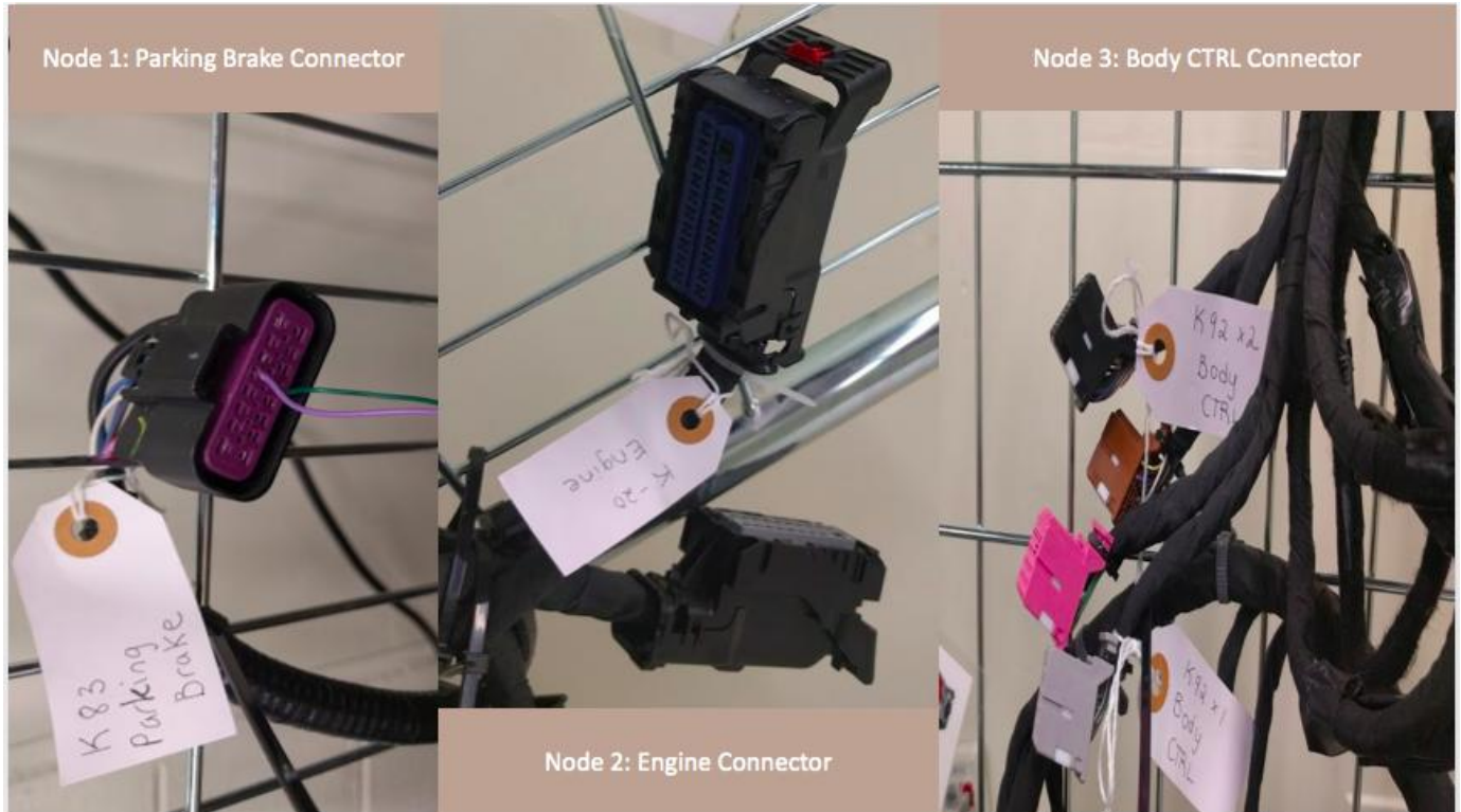
Figure 4.7: Close up of CAN Nodes available on the CAN Harness
