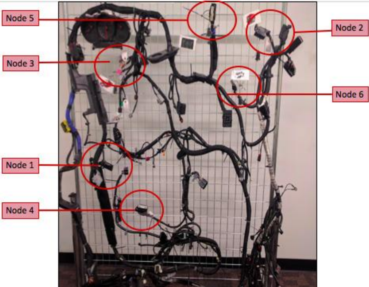
Figure 4.6: CAN Harness with 6 Nodes
