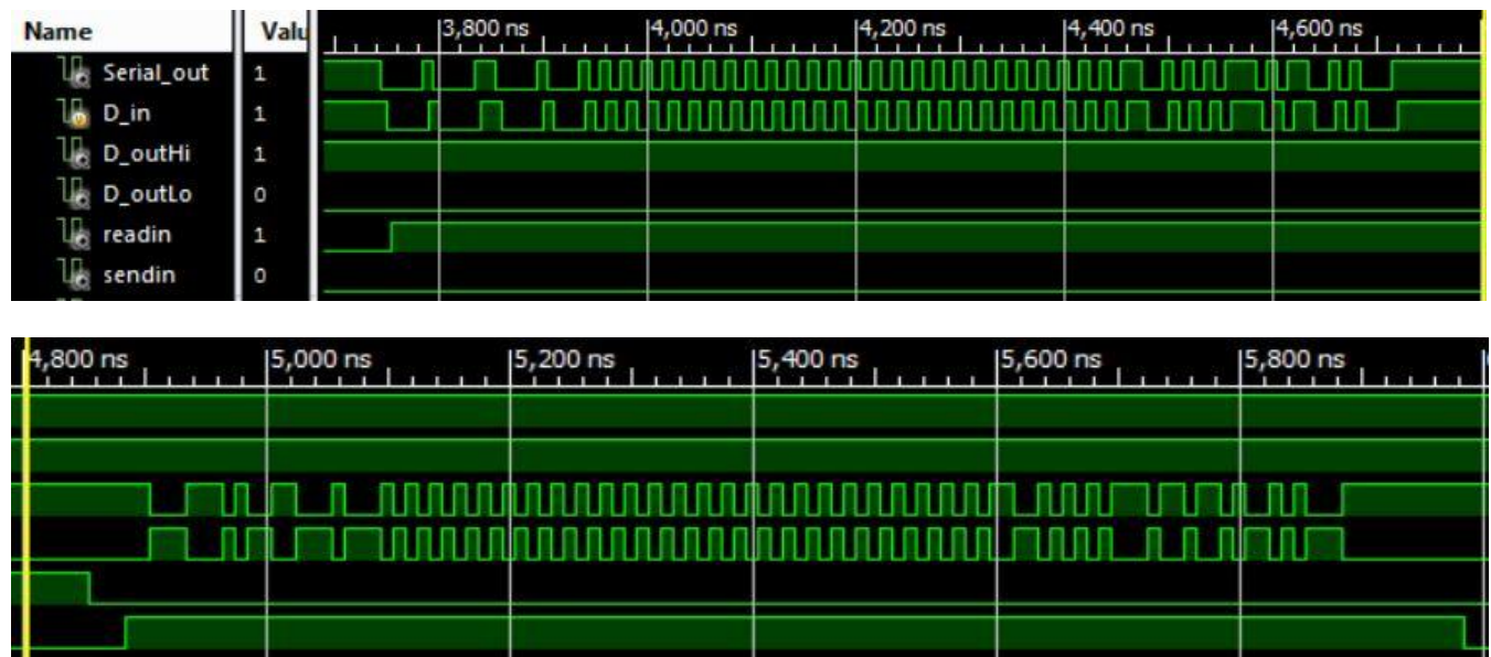
Figure 4.4: Read, perform operation on, and send message
