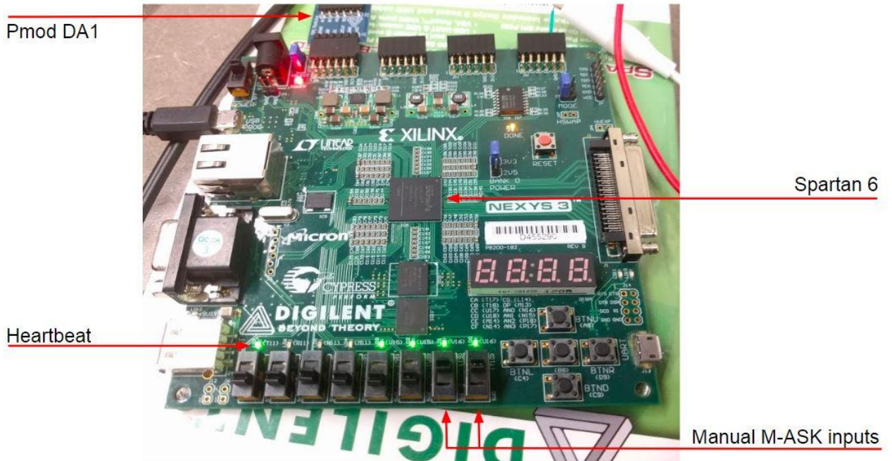
Figure 4.14: The Nexys 3 Spartan 6 FPGA with Pmod DA1 peripheral (AD1 not shown.)
