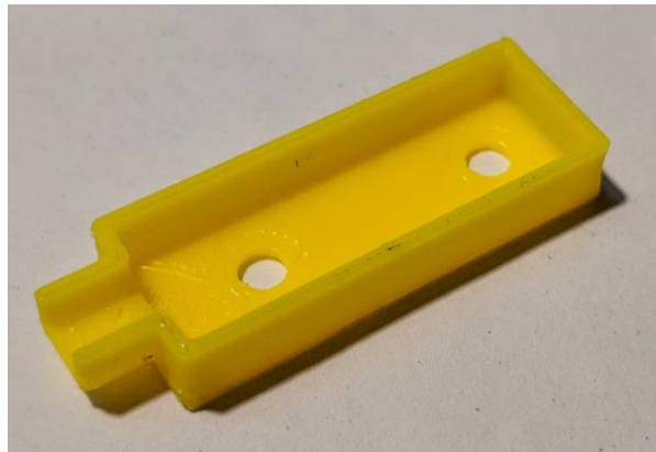
Figure 47: 3D Printed Encasement
