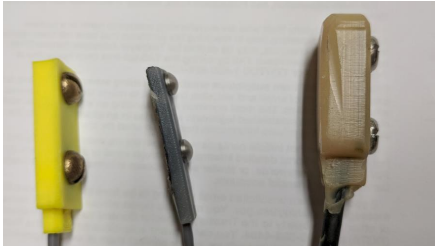
Figure 52: Side view of electrode versions (from right: 2002, 2015, 2018)
