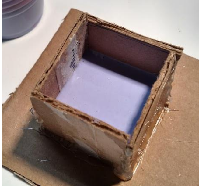
Figure 42: Poured Silicone Mold
