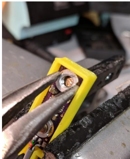
Figure 29: Using a Pair of Pliers to Grip the Modified Nut
