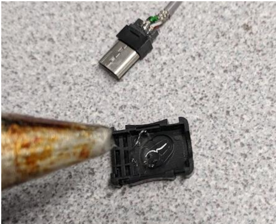
Figure 34: Hot Glue Applied to the Bottom of the Connector
