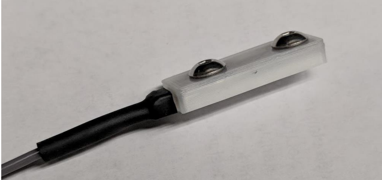
Figure 3: Electrode Amplifier Encasement
