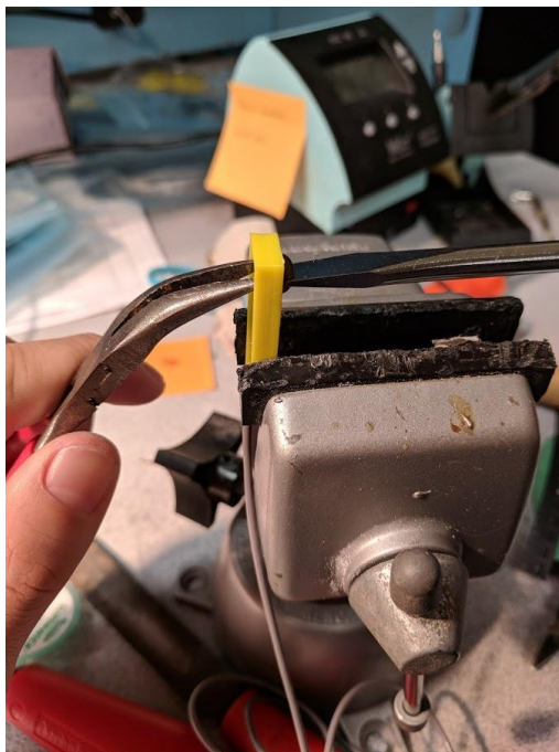
Figure 30: While Gripping the Nut with the Pliers, use a Screwdriver to Tighten the Bolt
