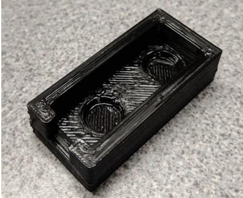
Figure 24: 3D Printed Silicone Mold
