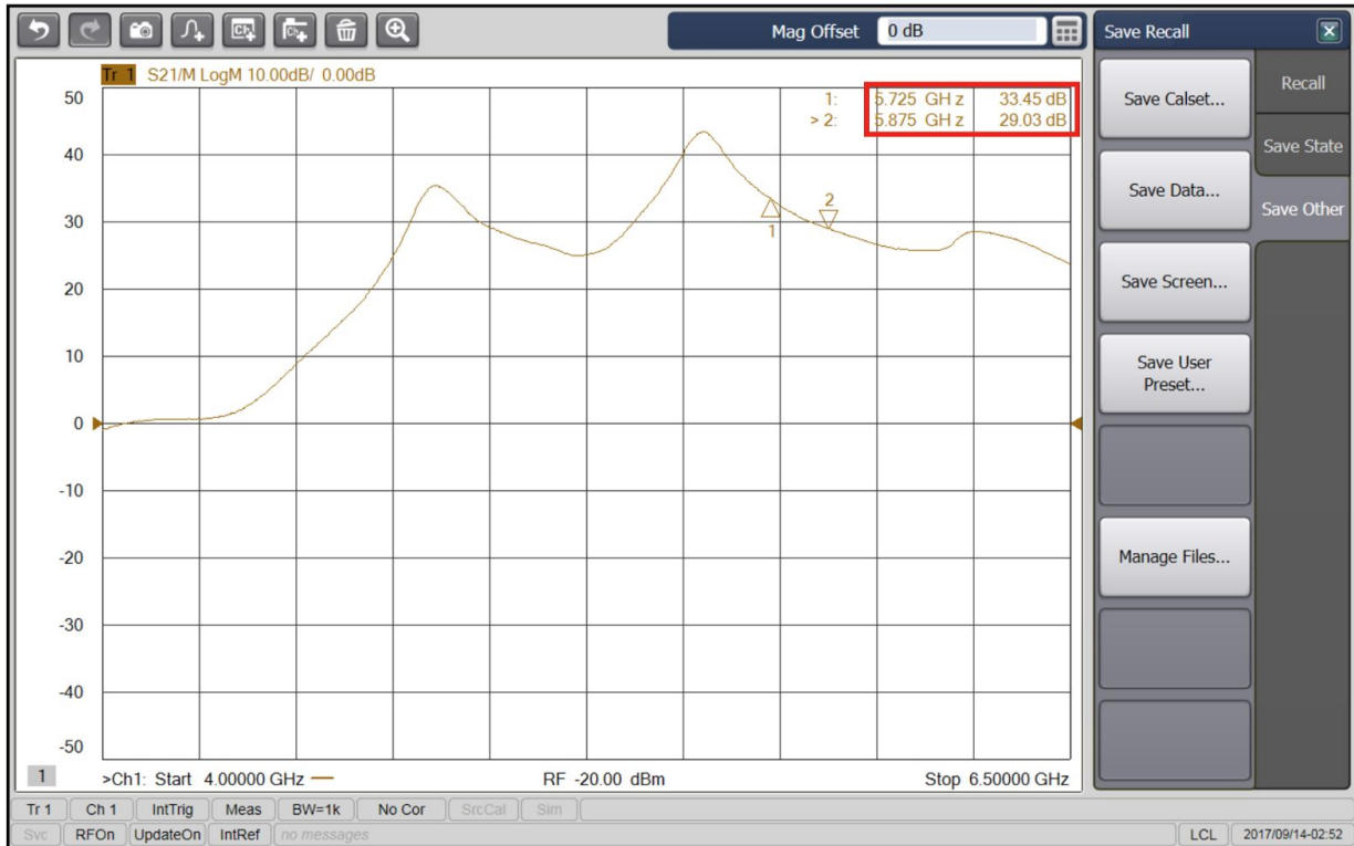
Figure 11: The modified amplifier swept (S21) from 4 GHz to 6.5 GHz showing the modification of stage removal and overall gain increase.
