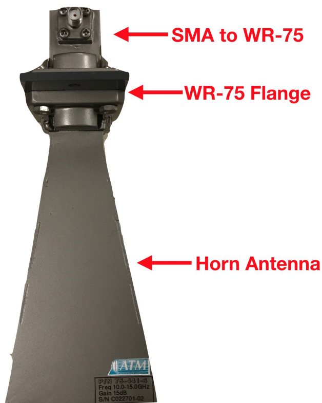
Figure 7: Pyramidal Horn Antenna on loan from WPI Professor Makarov. It came with a SMA to WR-75 waveguide adapter.
