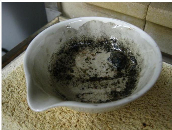
Figure 31: Paper Submerged in Molten Eutectic Salt
