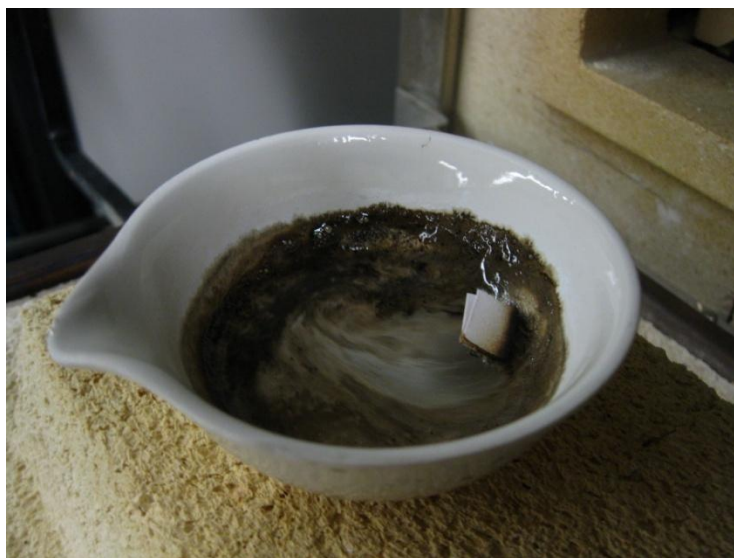
Figure 30: Paper Submerged in Molten Sodium Hydroxide
