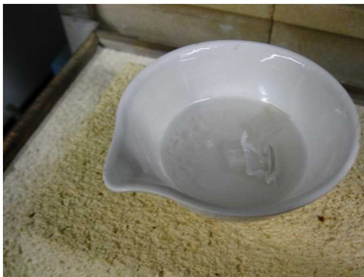
Figure 42: Plastic in Molten Potassium Hydroxide
