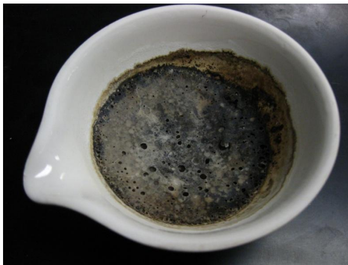
Figure 32: Hardened Bubbles from the Reaction of Paper Submerged in Sodium Hydroxide
