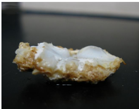
Figure 47: Plastic After Submerged in Molten Eutectic Salt
