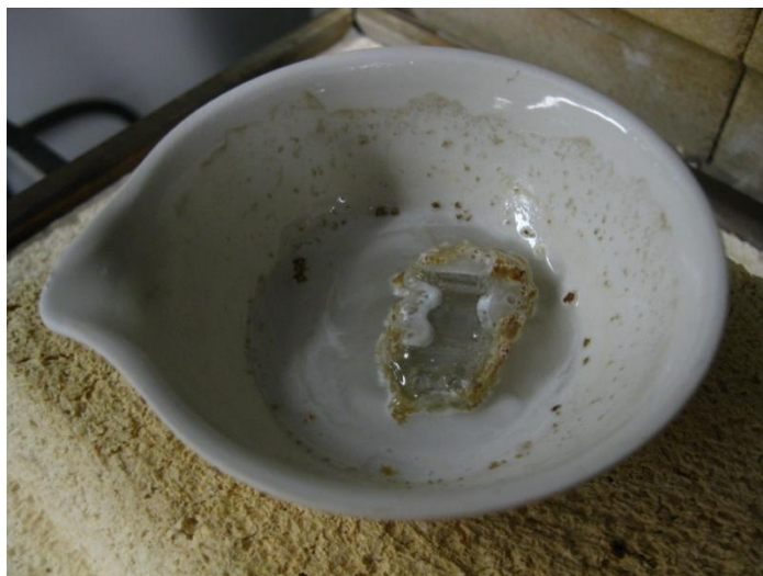
Figure 46: Plastic in Molten Eutectic Salt
