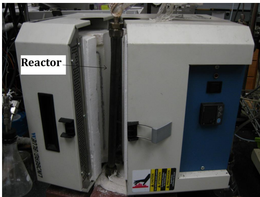
Figure 28: Lindburg/Blue Tubular Heater with Reactor
