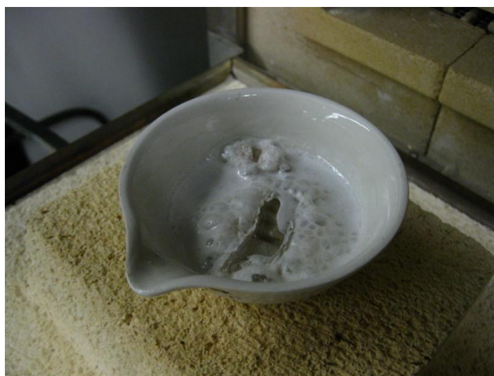
Figure 44: Plastic in Molten Sodium Hydroxide
