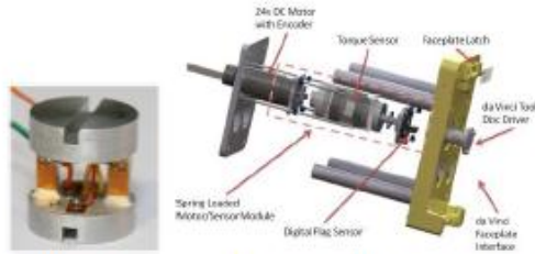
Fig. 3: Torque sensor and spring-loaded tool interface. The interface interacts directly with the standard da Vinci faceplate and is capable of manipulating the tool wrist while measuring the forces being applied to the tool tip.
