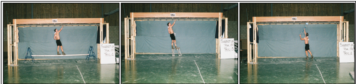
Figure 32 Trestle and stilts-mounted hand trowel use and trowel box use
