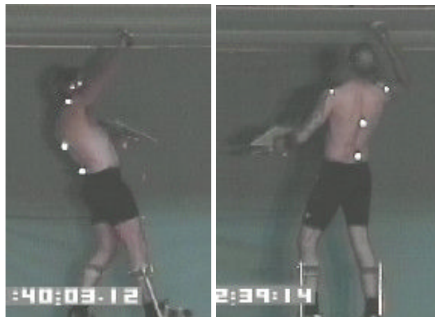
Figure 35 Reverse versus forward hand trowel use as viewed through the open side of the wall & ceiling frame.
