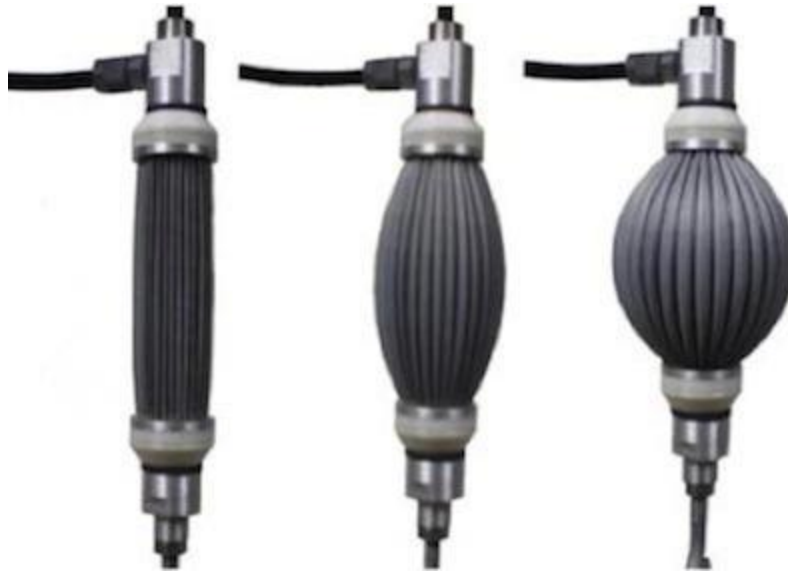
Figure 10: Pressurization of McKibben Muscle.
