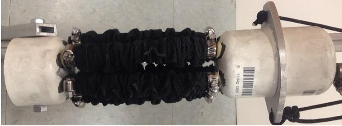
Figure 15: Final hydro-muscle construction. Both the prototype and final muscle fiber designs were utilized in the final robotic construction.
