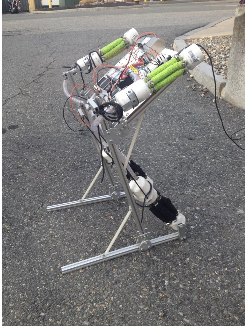
Figure 18: Iteration of the final construction with the prototype muscles used on top and the more powerful muscles used beneath.
