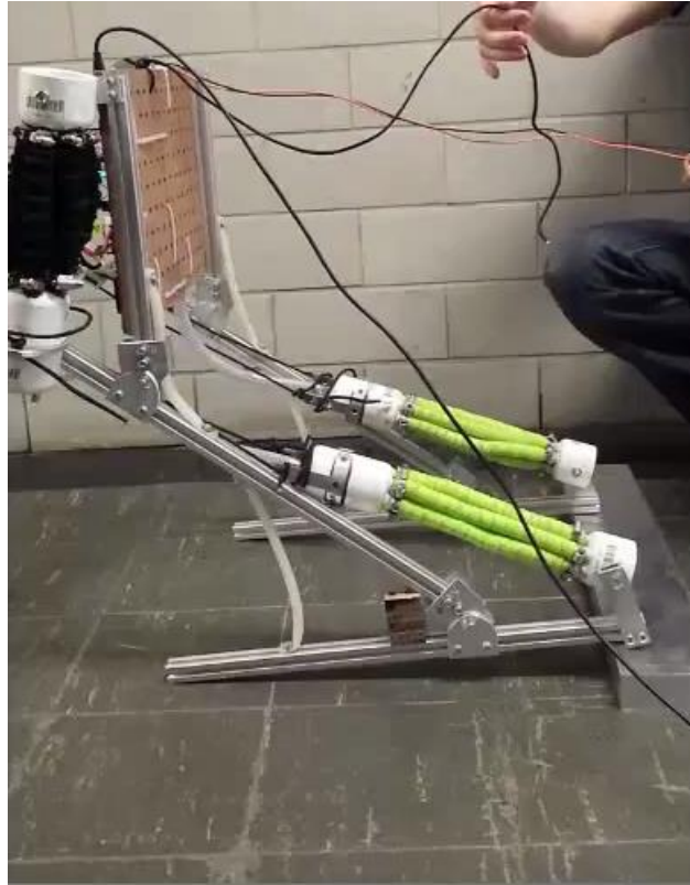
Figure 22: Iteration of final design in pressurized state, ready to perform a jump.
