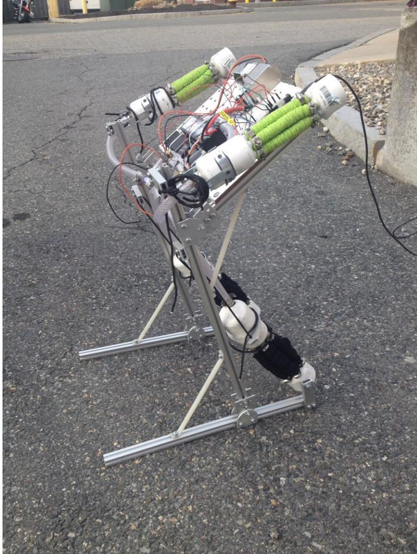
Figure 6: The skeleton of the robot allows easy adjustments of all leg lengths, pivot points, muscle attachment points, and center of mass adjustments.
