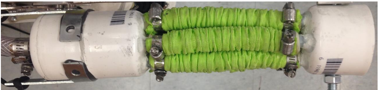
Figure 14: Prototype muscle fiber. After testing the prototype muscle fibers, it was decided to use larger tubing to increase the total force output.
