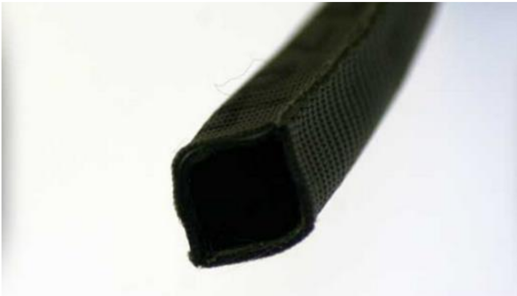
Figure 13: Nylon tubular webbing serves as the sheathing that constrains the elastomeric tubing in the hydro-muscle construction.
