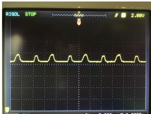
Figure 18: The Voltage across a Photoresistor in the Pickup as the String Below it vibrates
