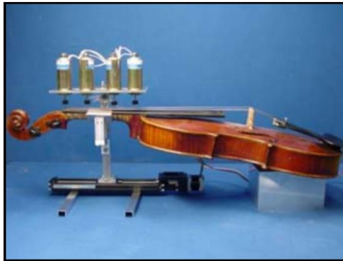
Figure 4: Shibuya Labs Prototype for Pitch Changing in a Violin Playing Robot[8]
