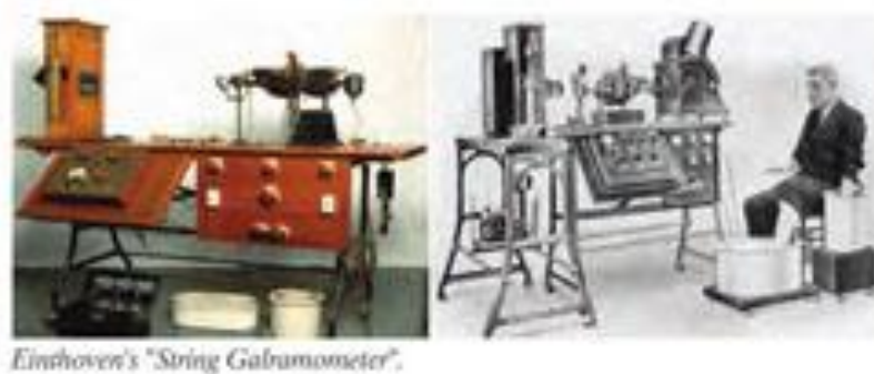
Fig. 3: Einthoven's "string galvanometer" used for his electrocardiogram work (Ball, 2010)
