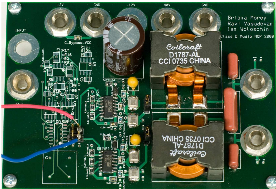
Figure 5.14: Populated Second Revision Printed Circuit Board
