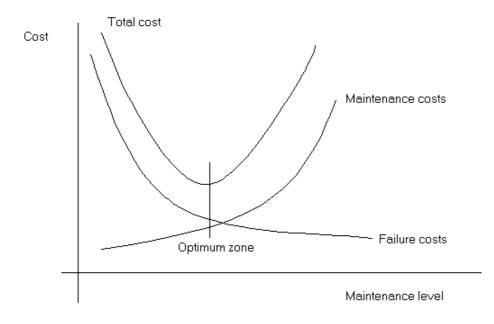
Figure 3.1: Maintenance and failure cost
