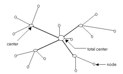
Figure 6.1: Two-level constrained hierarchical multicast tree
