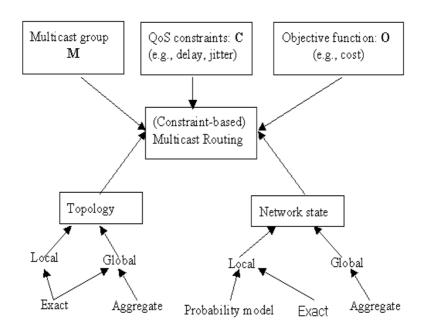
Figure 6.2: The various components in multicast routing
