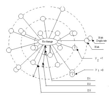
Figure 3.7: Network architecture for the simplified practical model (SPM)
