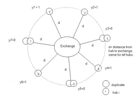
Figure 3.4: Network architecture for the simplified model (SM)
