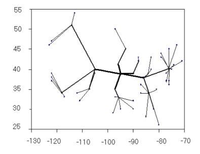
Figure 6.7: Three-level hierarchical multicast tree
