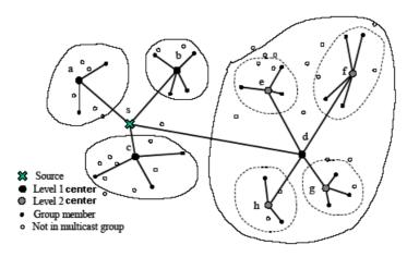
Figure 6.4: Forming multicast tree using clustering
