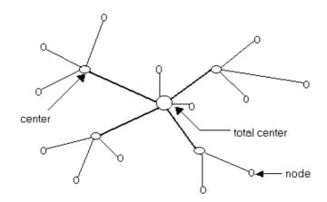
Figure 5.2: The two-level hierarchical tree topology
