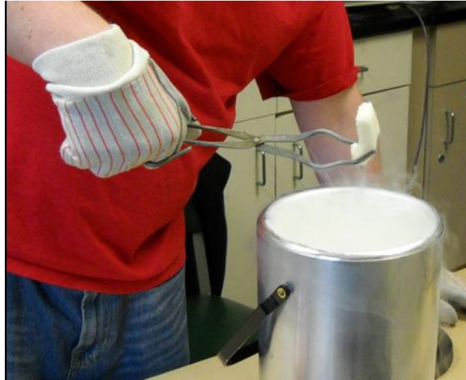
Figure 14 - Freezing Bread Samples with Liquid Nitrogen
