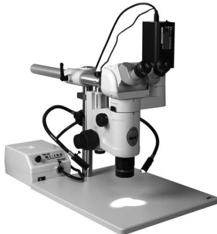
Figure 6 - Nikon SMZ 1500 with Camera Attachment
