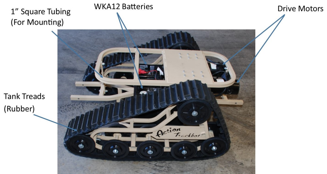
Figure 5: This is a labeled picture of the specific Action Trackchair platform provided to the team. It shows the location of the motors and the batteries.
